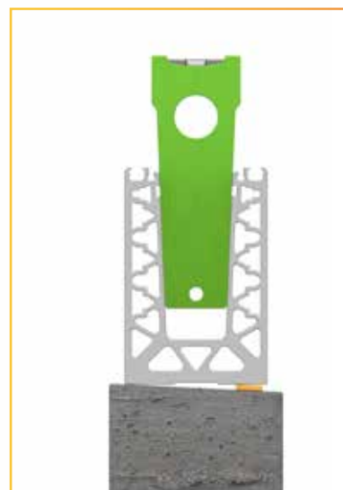
Figure 2 – instalation with shims
